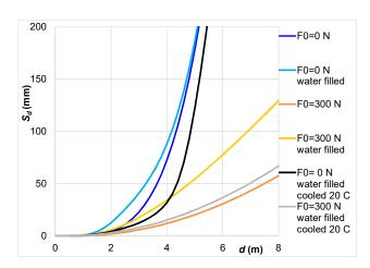
Figure 6. Example of Sag  $S_d$  as a function of span d for tensile force 0 N and 300 N on a 30/26 mm duct during hanging and how this is influenced by filling and cooling by  $\Delta T$  of 20 °C with water
