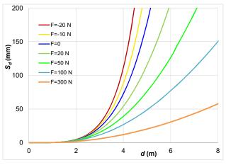
Figure 4. Sag  $S_d$  of the 32/26 mm duct as a function of span d for different forces.
