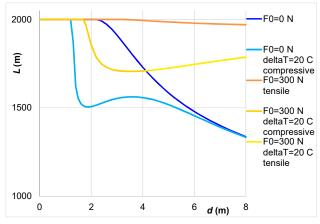
Figure 7. Example of blowing length *L* as a function of span *d* for a 20 mm cable in the 32/26 mm duct for the cases of Figure 5
