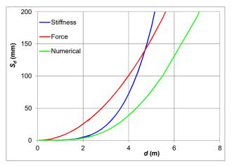
Figure 3. Sag  $S_d$  of the 32/26 mm duct as a function of span *d* for stiffness domination ( $S_{dB}$ , no force) and for force (50 N) domination ( $S_{dF}$ , zero stiffness). For both effects the numerical solution  $S_d$  of (A5) is given.
